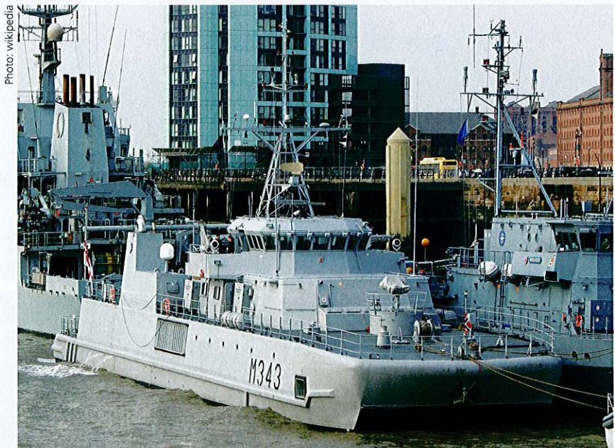
The Kvaerner Mandal-built OKSOY and ALTA Class MCMV catamarans were commissioned from 1994 and constituted the RNoN's first attempt to operate naval vessels incorporating surface effect technology.
