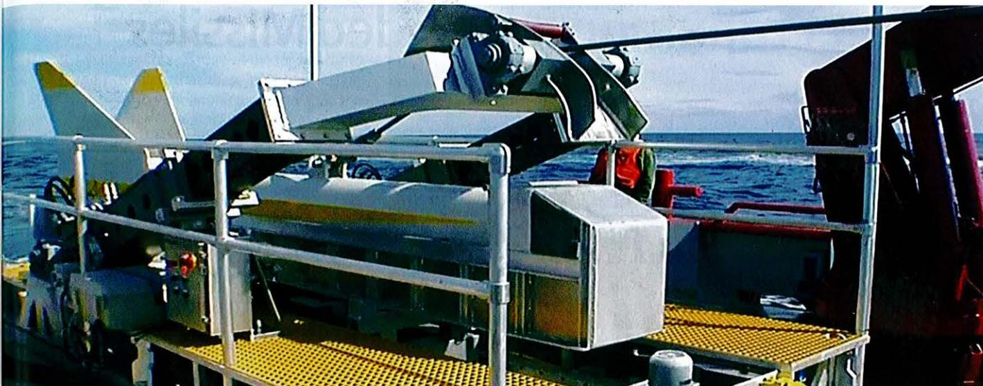
**The Variable Depth Sonar (VDS) from Raytheon is part of the LCS ASW Mission Package selected for both the FREEDOM and INDEPENDENCE Class vessels.**
