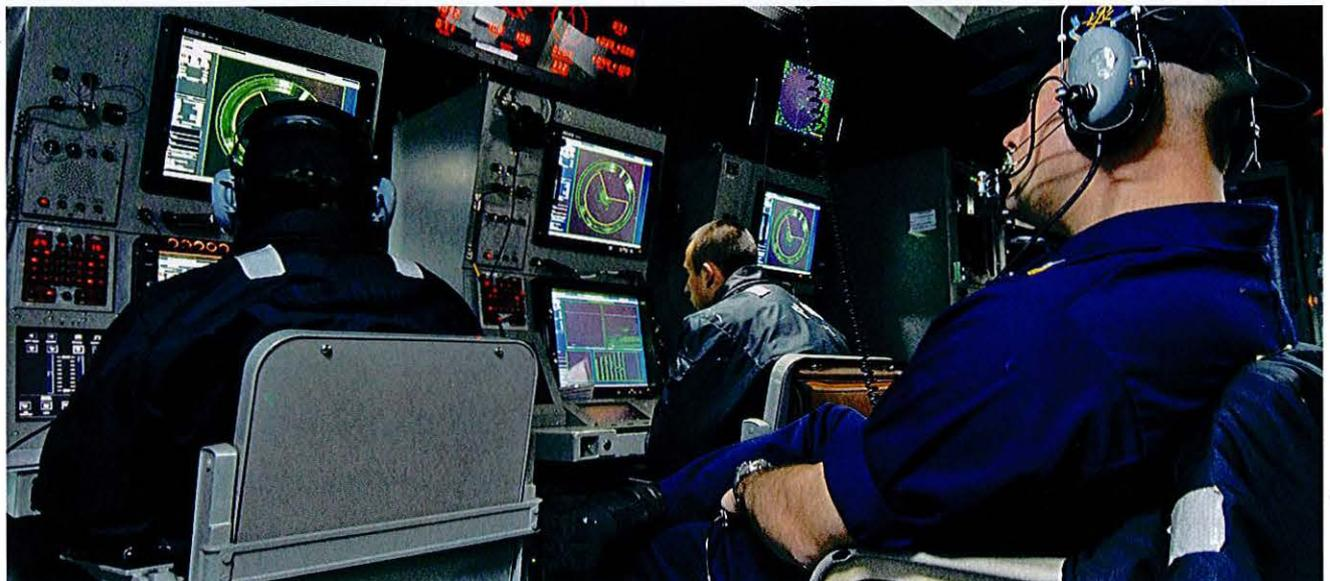
**Lockheed Martin's AN/SQQ-89V is the primary ASW system for the US Navy's surface combatants. Shown here are the consoles on board the ARLEIGH BURKE Class destroyer DDG 92 (USS MOMSEN).**
